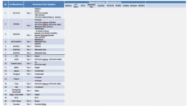
Table 8: Power Transistor Modules used in Automotive Motor Inverters and DC-DC Converter
